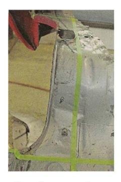
4.) Carefully cut along these lines removing a small section of outer frame rail, and a small section of the lower control arm mount. (See photo)
