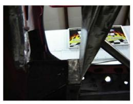
7.) Finish cut the rest of the old inner wheel-house out and grind smooth all the seam sealer.
