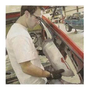
3.) Start laying out your cut lines for the mini tubs, lay out the rear cut lines by running a straight line from the back of the passenger side wheel- house to the back of the driver side wheel house.
